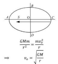
Hence, larger the distance, smaller the orbital velocity. At point *C* distance from sun is maximum, hence orbital velocity is lowest. At point *A* distance from sun is minimum, hence orbital velocity is maximum.
